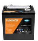
LTL series is specially designed for frequent discharge deep cycle application. By using the specially designed active material, strong grids and thick plate construction, the LTL series battery offers reliable performance in high load situations and could provide competitive cycle performance. It is suitable for Electric Vehicle and Golf cart, Floor Machines, Forklifts, Aerial lifts, Robotics, Marine, RV, Mobility and Medical Equipment, and most outdoor application.
